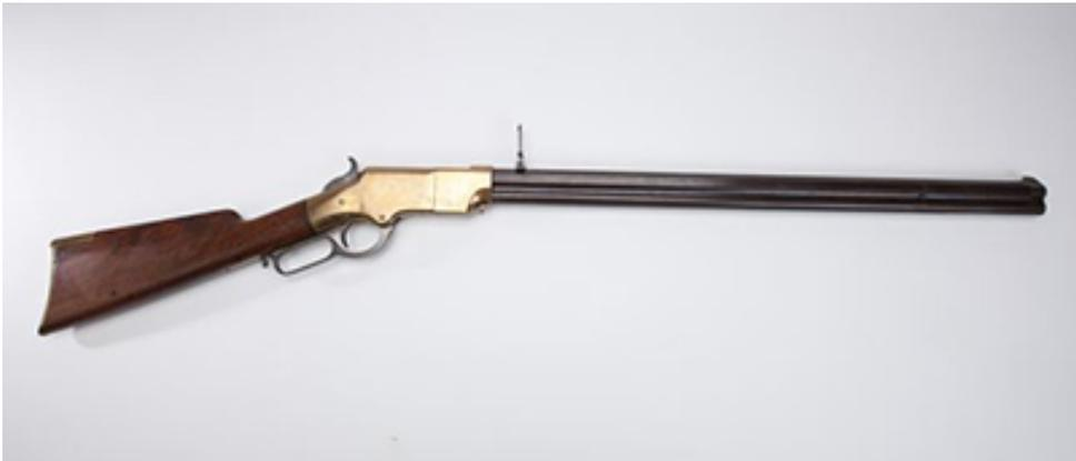
The [1860 Henry](#) lever action rifle. This specimen was manufactured 1864. The lever is the oval that attaches to the trigger guard. The oval and the guard move as a unit, swung down to eject, then up to reload. The pivot is at the top front of the trigger guard. The rifle is still in production today, with modifications for modern ammunition.
